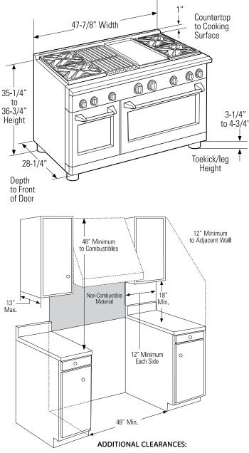
Allow 12" minimum clearance to an adjacent wall on each side.
