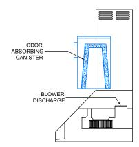
14) Move the canister all the way to the back and then lower the canister over the blower discharge. Shift the canister front to back and left to right to make sure that the blower discharge and canister have fully engaged.
