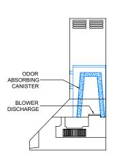
15) With the gasket side facing down, nest the smoke trapping filter element into the pocket that forms the top of the odor absorbing canister. The filter may have a rectangular base so rotate as necessary. Replace the duct cover front panel by aligning the snaps and pressing each snap into position.
