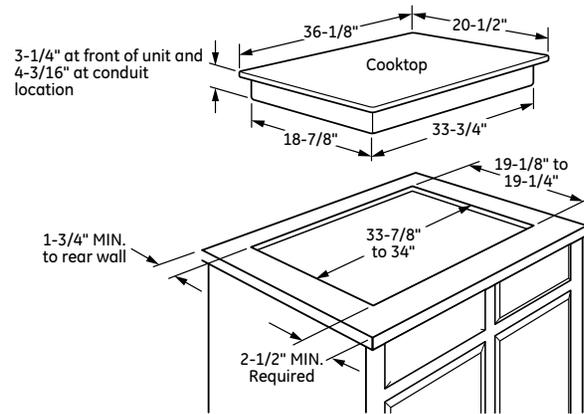
To insure accuracy, it is best to make a template when cutting the opening in the counter
