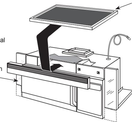
Filter Kit JX81D—Recirculating Charcoal Filter Kit To be used when the microwave oven cannot be vented to the outside.
